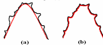
Fig. 1. Comparing the segmentation features of Fast Matching (a) with MR (b), where the black lines represent the object edge and the highlighted lines depict the segmented lines.
