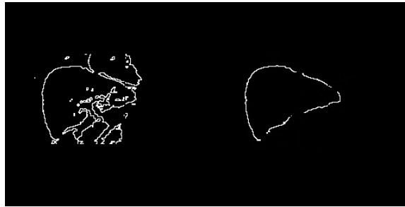
Fig. 2. Selection of the template image. (left) shape before refinement. (right) shape after refinement.
